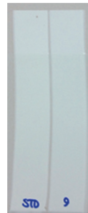
Fig. 5 Firing test of the standard (l.), and the new engobe formula (r.) for ceramic tiles
